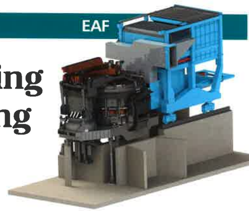
Fig 1 The EPC scrap pre-heater mounted on wheeled bogies moves to mate with the off-gas and wall charging port of the EAF
